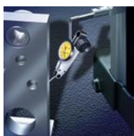
Perpendicularity using TESATAST
